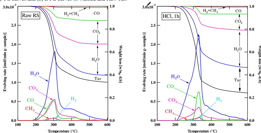
Figure 2. TG curve, gas formation rate and product distribution during the pyrolysis of raw of Raw-RS and HCl.
