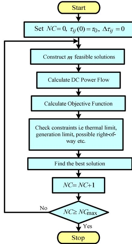
**Figure 4.** Flow chart of TEP-ACO algorithm.
