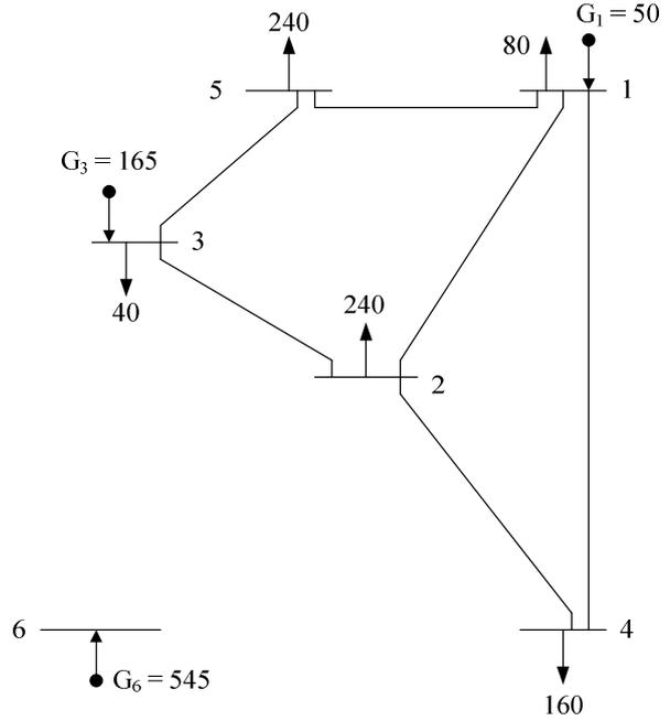
**Figure 5.** Initial configuration of Garver's 6-bus network.
