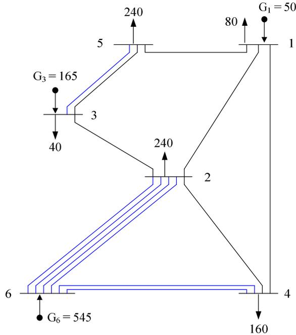
Figure 6. Optimal plan of Garver's 6-bus system.
