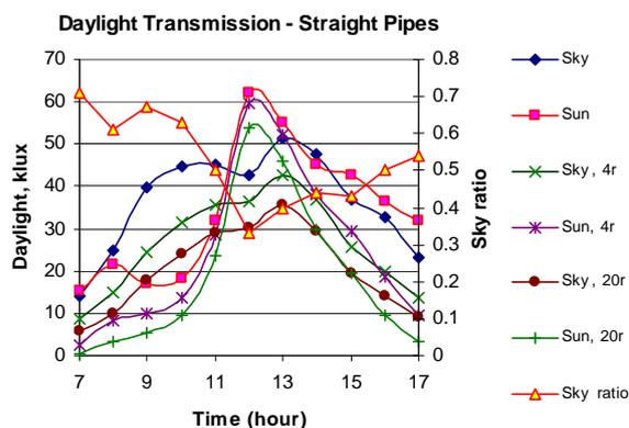
(a) Measured daylight and calculated transmitted daylight
