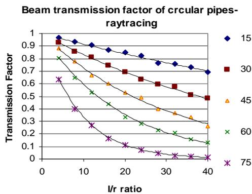
(b) Transmission functions calculated from raytracing.
