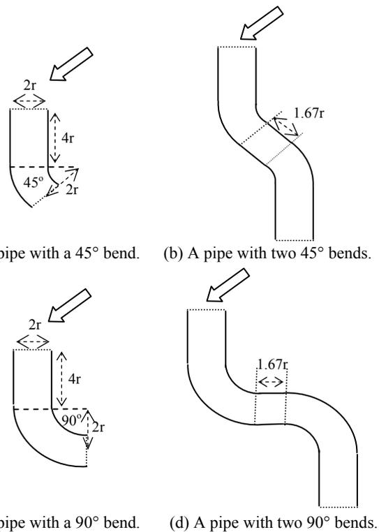
(a) A pipe with a 45° bend. (b) A pipe with two 45° bends. (c) A pipe with a 90° bend. (d) A pipe with two 90° bends.
