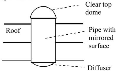
(a) Passive roof-mounted light pipe
