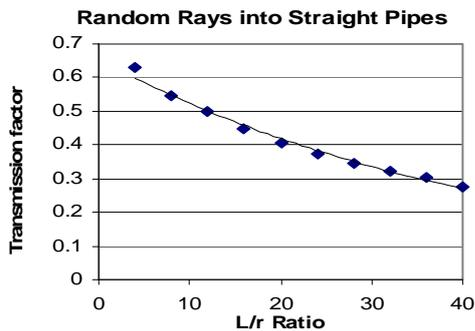
**Figure 5.** Graph of transmission factors for rays from Lambertian surface.
