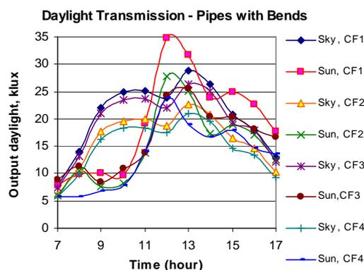
(b) Calculated daylight through pipes with bends.
