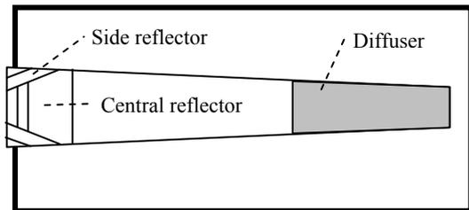
(b) Plan view of façade-mounted light pipe
