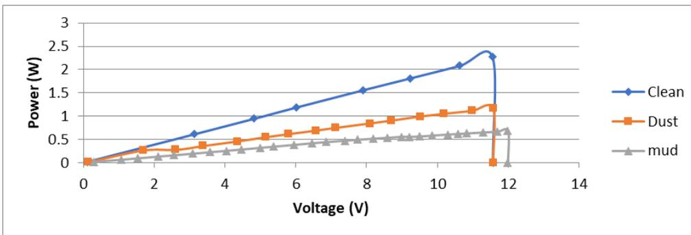
Figure 8. P-V characteristic of a PV cell with dust, mud and clean surface for irradiance of 466.4 W/M<sup>2</sup> for 30 cm.
