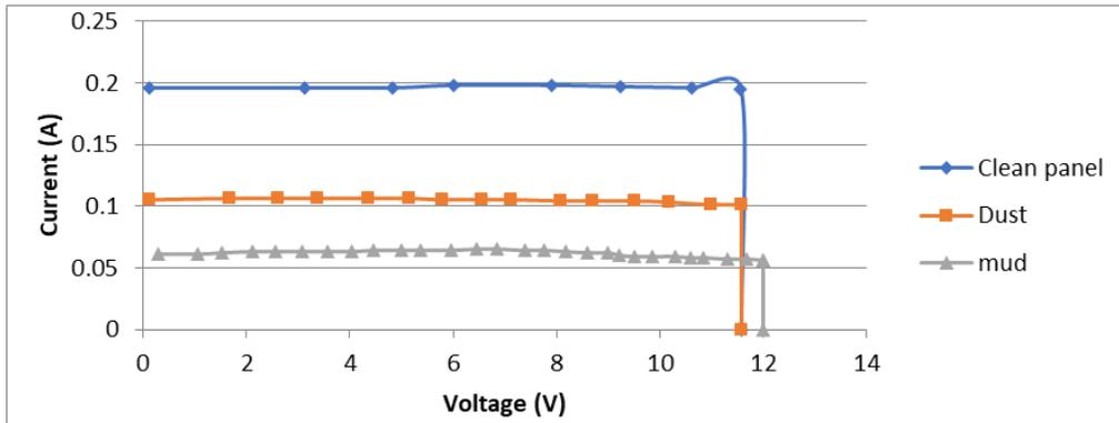
Figure 6. I-V characteristic of a PV cell with dust, mud and clean surface for irradiance of 466.4 W/M<sup>2</sup> at 30 cm.
