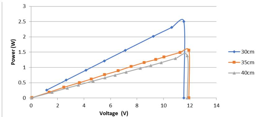
Figure 3. P-V characteristic of a PV cell at difference irradiance and height.
