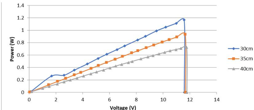
Figure 5. P-V characteristic of a PV cell at different irradiance and height.
