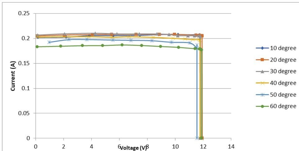
Figure 9. I-V characteristic of a PV cell with different tilt angles for irradiance of  $466.4 \text{ W/M}^2$ .
