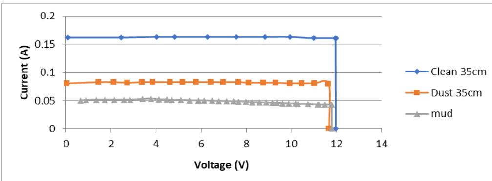
Figure 7. I-V characteristic of a PV cell with dust, mud and clean surface for irradiance of 402.8 W/M<sup>2</sup>.
