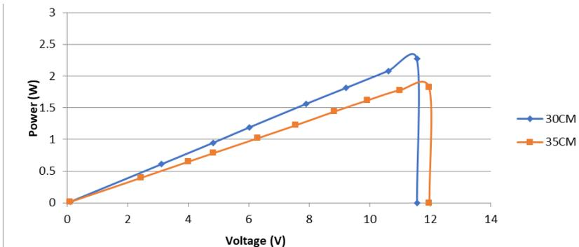
Figure 4. P-V characteristic of a PV cell at difference irradiance and height.
