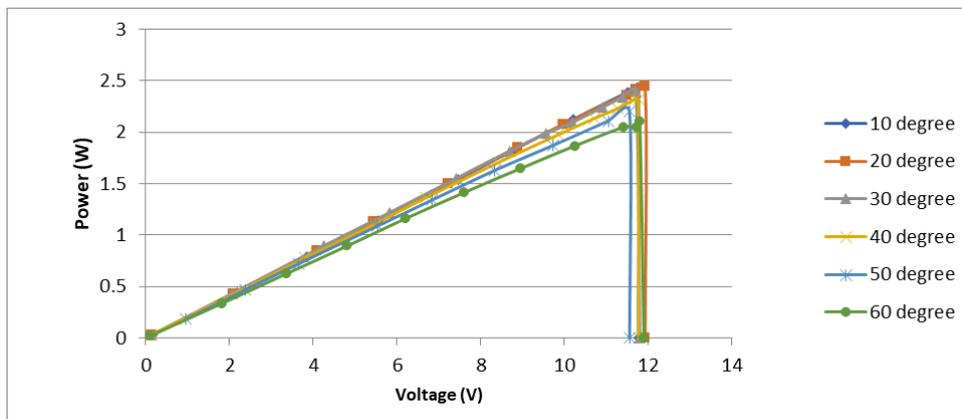
Figure 10. P-V characteristic of a PV cell for irradiance of  $466.4 \text{ W/M}^2$  with different tilt angle.
