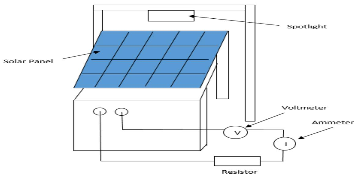
**Figure 1.** Block diagram representing the schematic of the system with the halogen lamp.
