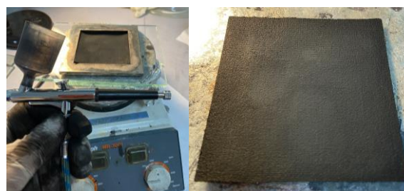
Figure 5. Spraying technique of catalyst material on GDL.
